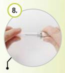
Connect peristaltic pump or diluter using Bag Connector, then open clip to allow media to flow.
